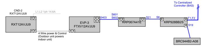
Div 15 : Low Voltage control wiring 18 AWG 2-conductor stranded non-shielded (unless otherwise noted)
