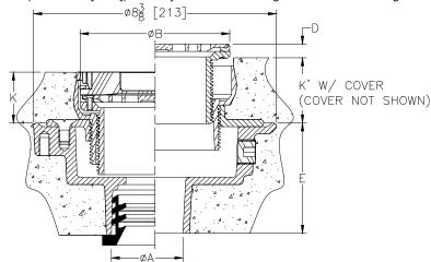
Note: Minimum K Dimension is only possible with -LR Option when using 6" [152] or 8" [203] Strainer
