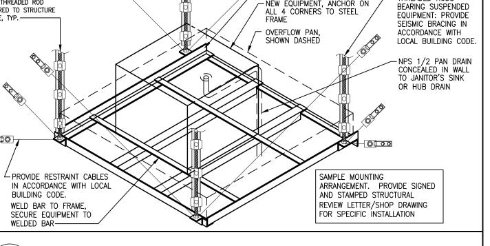
HOT WATER TANK SUPPORT DETAIL
