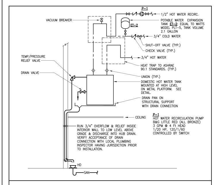
HOT WATER TANK (WH-2) DETAIL M3 / SCALE: NOT TO SCALE
